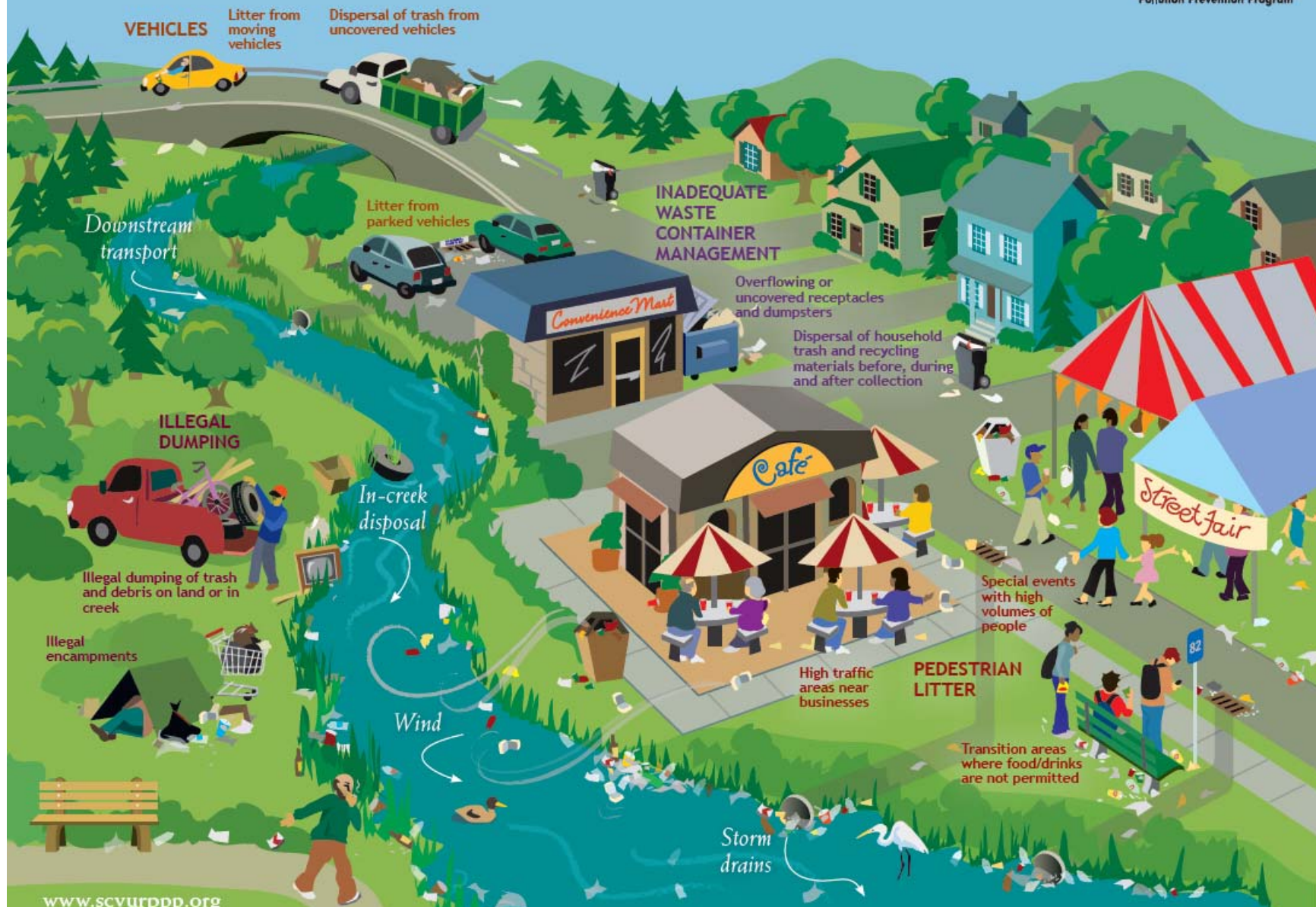
Figure 1. Potential trash sources and transport pathways to urban creeks. Source categories include pedestrians, vehicles, waste containers and illegal dumping. Stormwater conveyance systems, wind, direct disposal and downstream transport are transport pathways.
